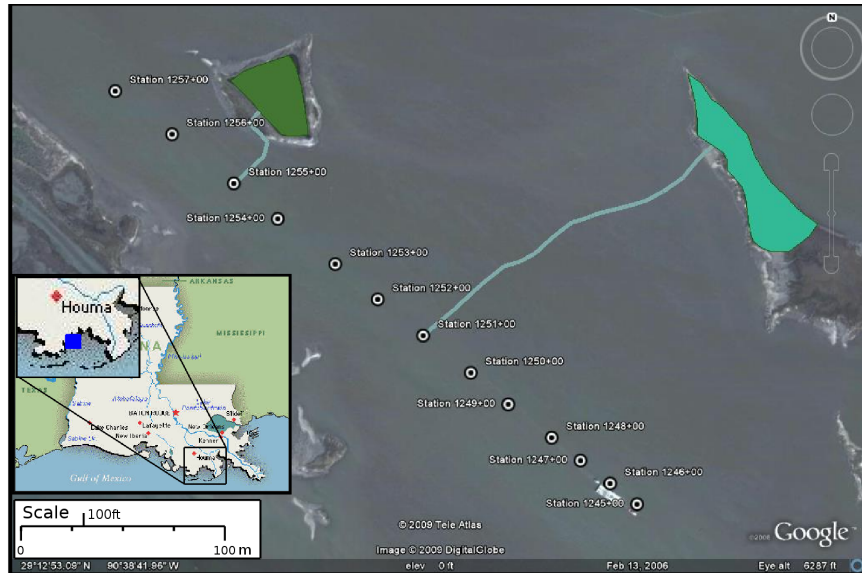
Figure 12: Example application pipeline dredge project components.
