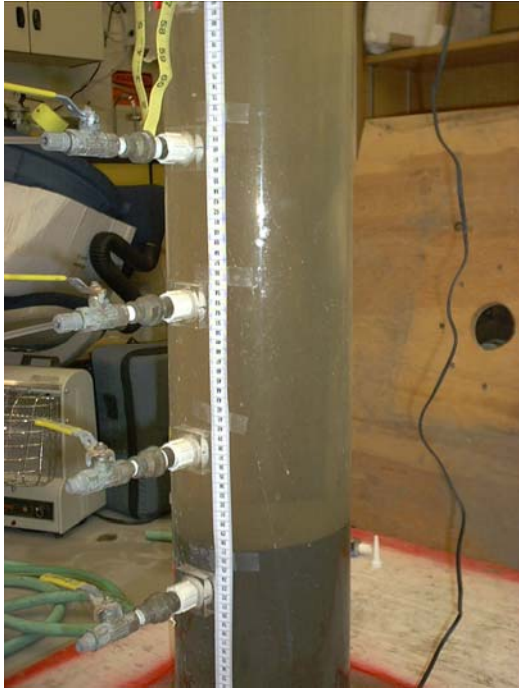
Figure 1. Zone settling column test and typical
