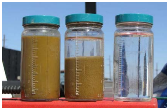
Figure 7. The raw dredged sample (left) was conditioned with 66-ppm of Solve 9330 (center). The filtrate collected from the geotextile containers is on the right.
