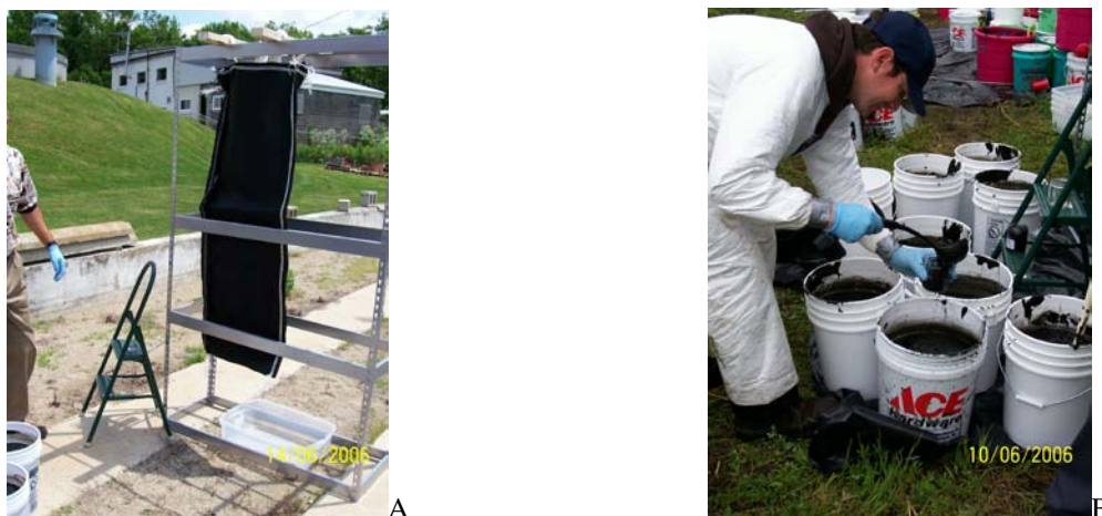
Figure 1. A) Geotextile hanging bag dewatering performance trial. B) Sediments were collected for analytical testing (e.g., contaminants, percent dry weight solids).
