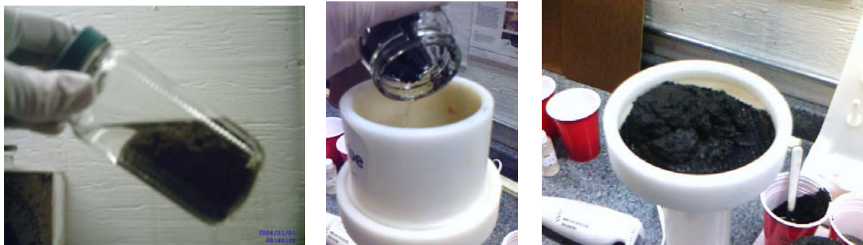
Figure 5. Dredge residual sample conditioned with 50-ppm Solve 9330 (left). A 150-mL conditioned sample was poured through a GT500D filter (center). Residual cake remaining on the filter after 60 minutes (right).
