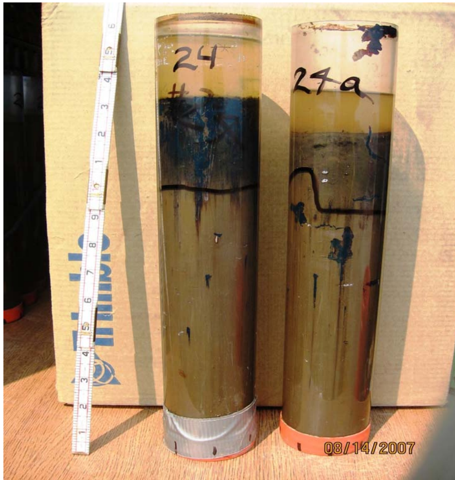
Figure 5. Typical NDR Cores. Note the contrast between the dark brown and black dredge residue and the light brown underlying native sediments.
