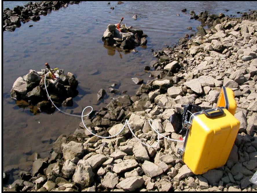
Figure 9. Flux chamber set (2008).
