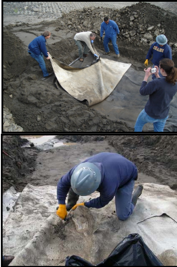
Figure 11. Exhumation of the “test” Reactive Core Mat® for sampling (2006).
