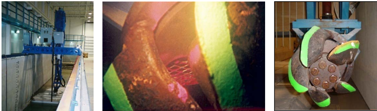
Figure 4. Dredge carriage (left), screened suction inlet (center), and cutter (right).
