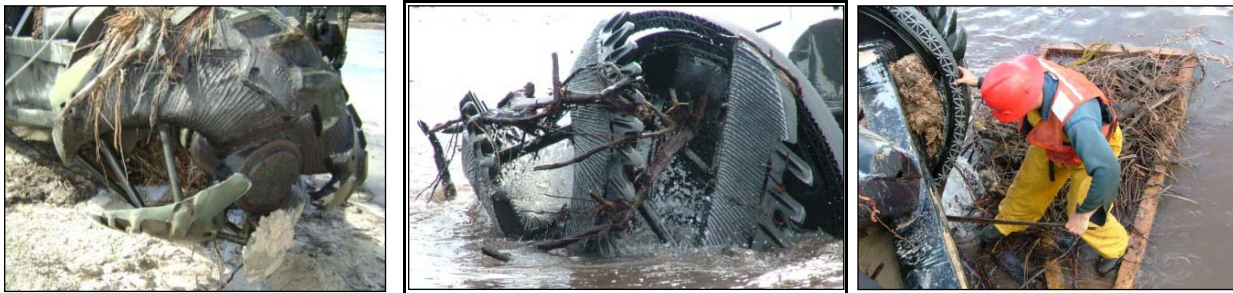
Figure 2. Roots in suction mouth (left), cutter (middle) and being cleaned from cutter (right) (Courtesy of Manson Construction Co.).
