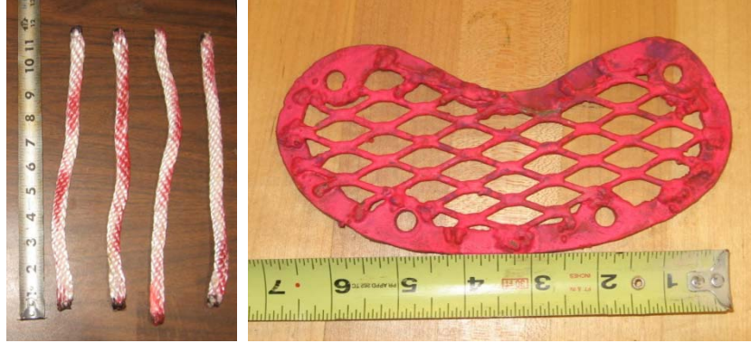
Figure 5. Rope used to simulate roots (left) and suction inlet screen (right). The scales are in inches which may be converted to centimeters by multiplying by 2.52.
