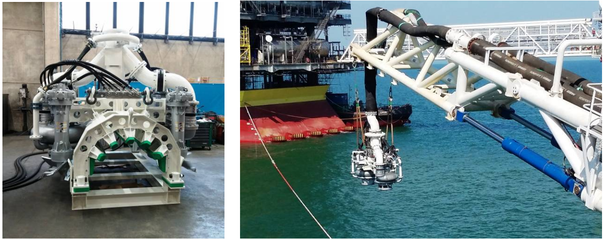
Figure 32 and 33. Dredging tool for submerged pipeline maintenance
