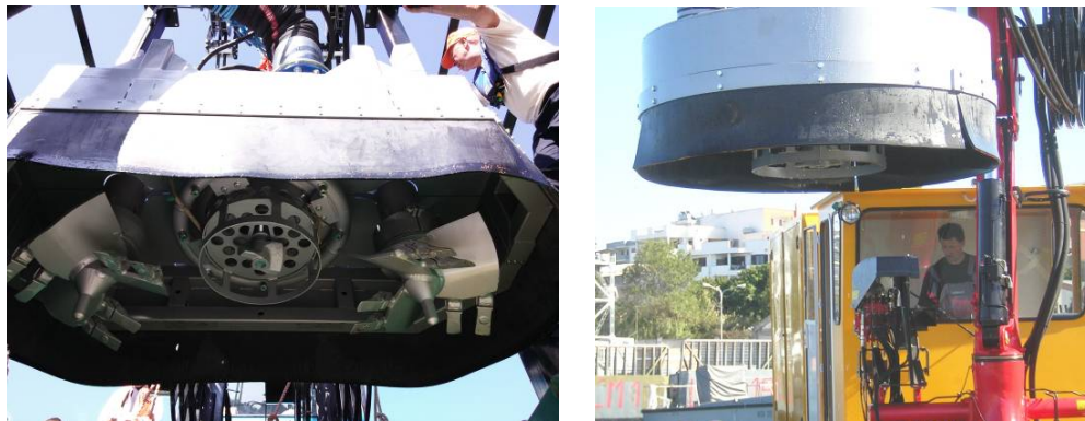
Figure 8 and 9. Anti-turbidity bells.
