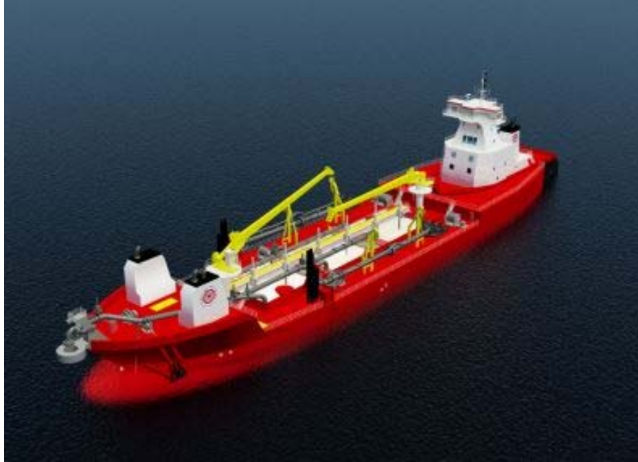
Figure 2. GLDD ATB hopper dredge.
