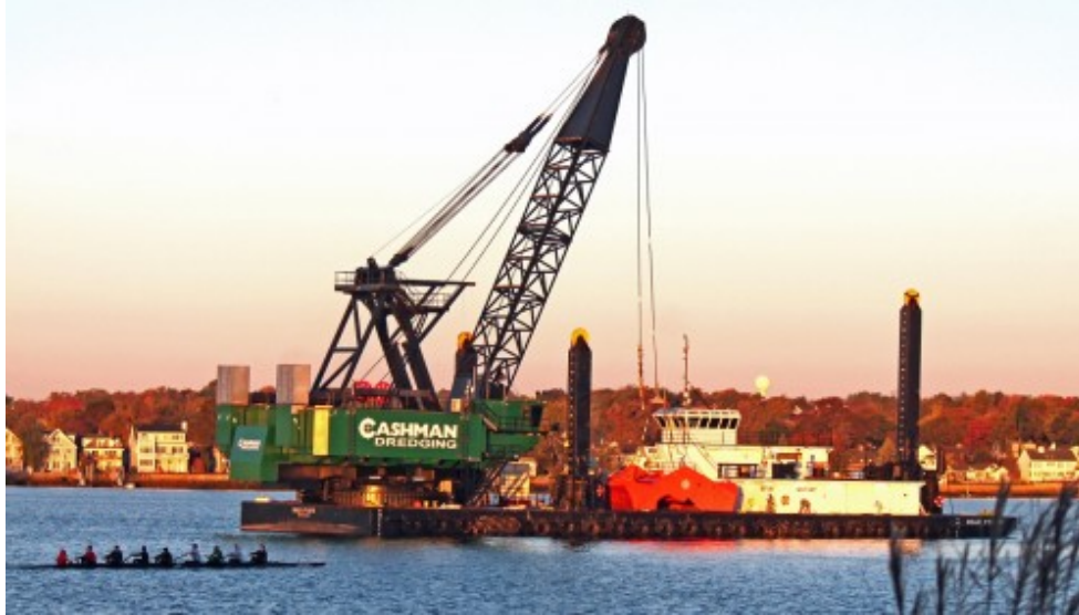
Figure 4. Cashman clamshell dredge. (Source: http://www.norwalkcove.com/?p=2142 )
