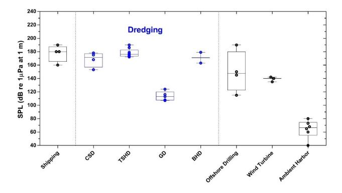
**Figure 2. Summary of non-impulsive underwater SPLs by sound source.** Dredge-induced sounds (blue) include: cutter suction dredge (CSD); trailing suction hopper dredge (TSHD); grab dredge (GD [recorded 158 m from source]); and backhoe dredge (BHD). References: shipping (OSPAR 2009a; Reine et al. 2014b; Merchant et al. 2016); offshore drilling (Richardson et al. 1995; OSPAR 2009a); wind turbines (OSPAR 2009a); ambient harbor (Wenz 1962; Reine et al. 2014b; Merchant et al. 2016).
