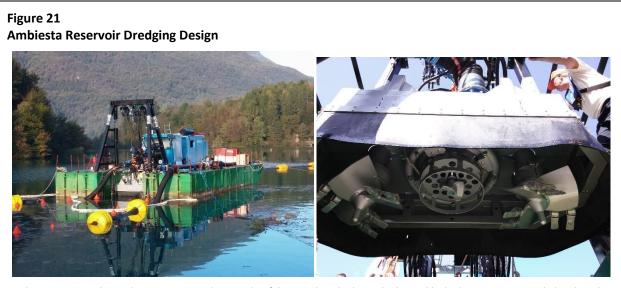
Dredging system used at Ambiesta Reservoir; photographs of the complete dredge and submersible dredging pump anti-turbidity shroud Source: Dragflow
