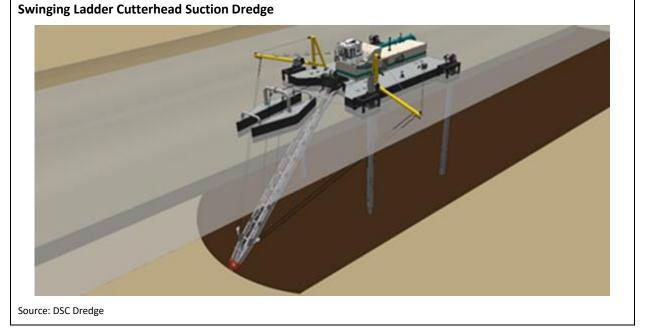
Hydraulic dredges are characterized by their use of centrifugal pumps to remove bottom material by entraining it with water at the dredge suction mouth to create a slurry (solids and water mixture) that is
