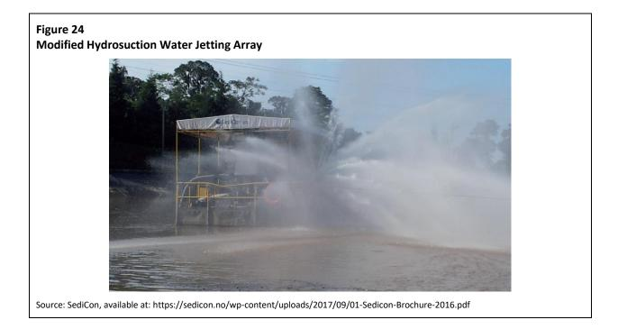
*Water Injection Dredge:* The water injection dredge (WID) is a dredging technique primarily used in navigation dredging in which a dredge vessel pumps water into channel bottom sediments at low pressure and relatively high-volume flow rates. This dilutes and fluidizes the sediments, creating a near-bottom layer (density current) with higher density than the surrounding water. This layer is then transported downslope by
