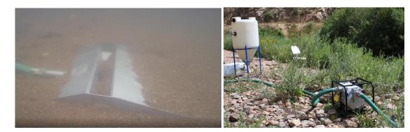
Sand and gravel being deposited into a collector prior to being pumped to shore and volumetrically measured in production time trials Source: Streamside Systems LLC
