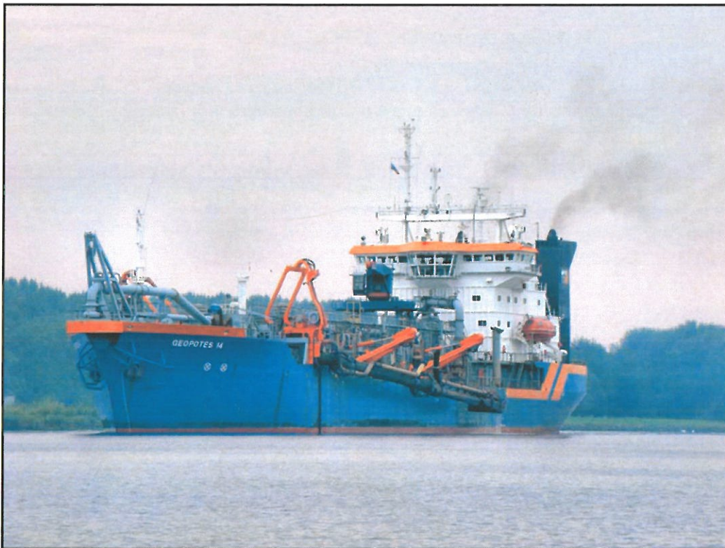
Trailing Suction Hopper Dredge "Geopotes" (Netherlands)
