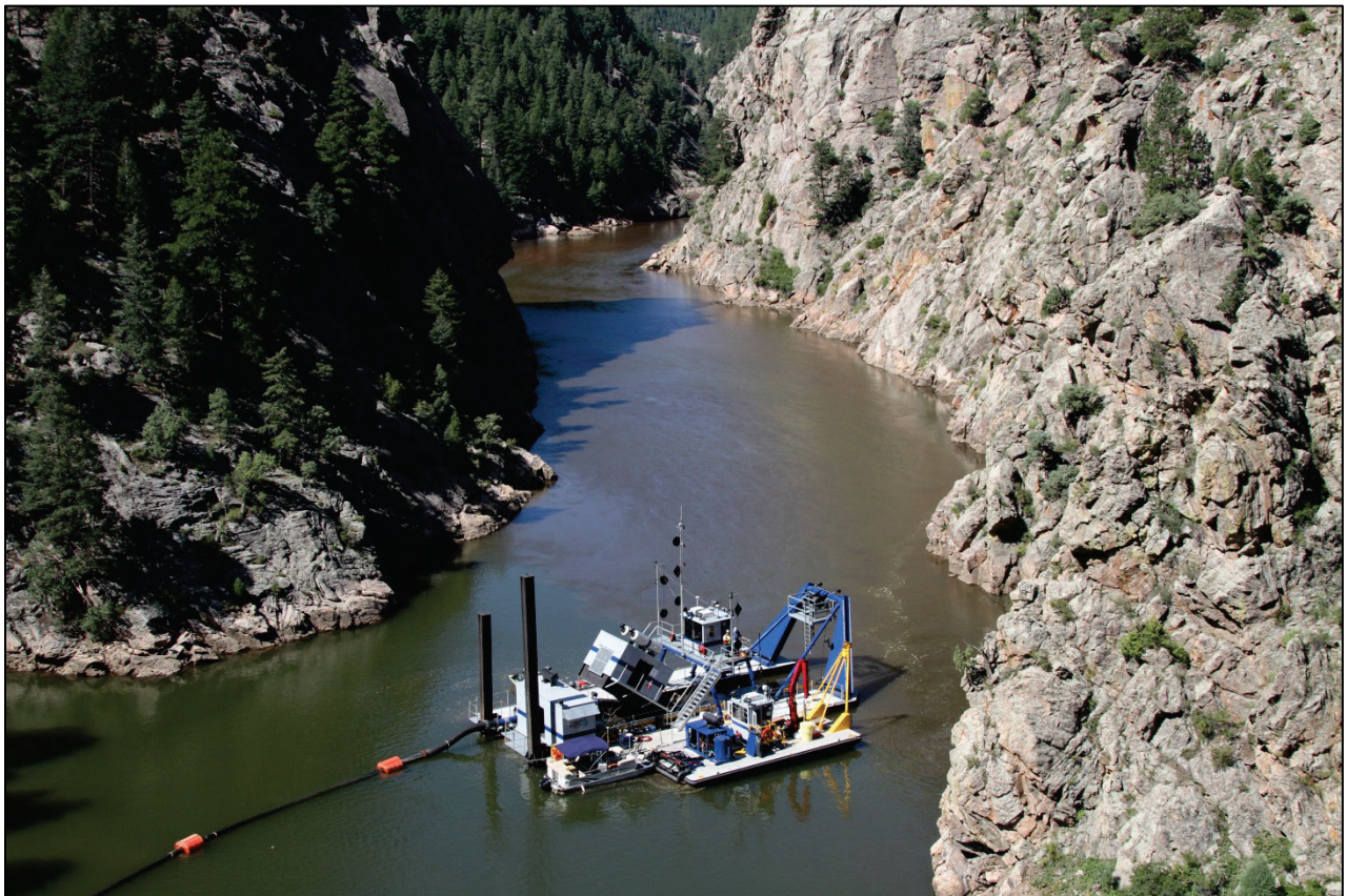
Sevenson's 16-Inch DSC Marlin Dredge with Dredge Tender (Photo Courtesy of Sevenson)
