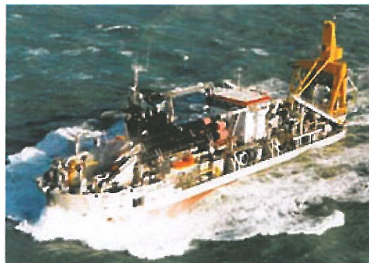
Figure 2. J.F.J. De Nul Self-Propelled Cutter Suction Dredge (Courtesy of Jan De Nul).
