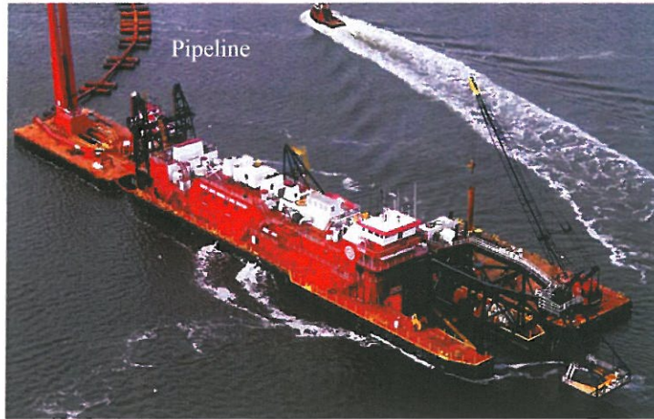
Figure 1. Cutter Suction Dredge Texas (Courtesy of Great Lakes Dredge & Dock).
