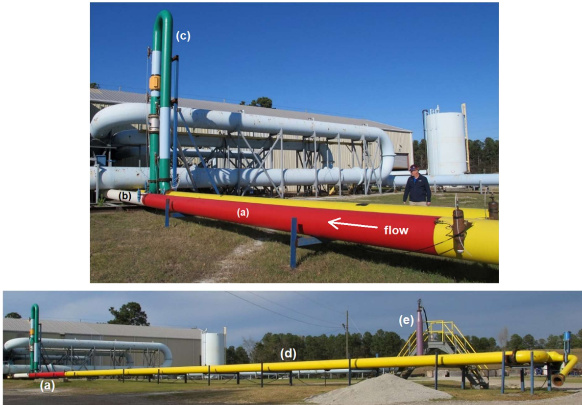
Figure 3. 489 mm system showing: (a) first half of measurement section (red), (b) second half of measurement section - partly hidden, (c) inverted U-loop for SG measurement with magnetic and ultrasonic flow meters, (d) entrance section (yellow), (e) de-aeration stack.
